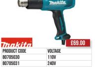
Makita HG5030K Heat Gun 110V Heat Settings2 Temperature 110V400 - 550 °CTemperature 240V350 - 500 °C Air Flow 110V200 - 400 litres/ min Input Wattage 110v1,300 w Net weight 0.56 kg
