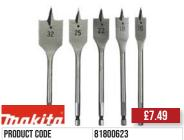
A flat bit with a grooved head for improved centering and discharge and a hexagon shank that prevents chuck slippage. Improved centring and discharge Ideal for most types of wood, hard or soft. Features: Grooved head, Hexagon shank, Contains: 5 - Flat bits, 150mm(L):16,18,22,25,32mm.
